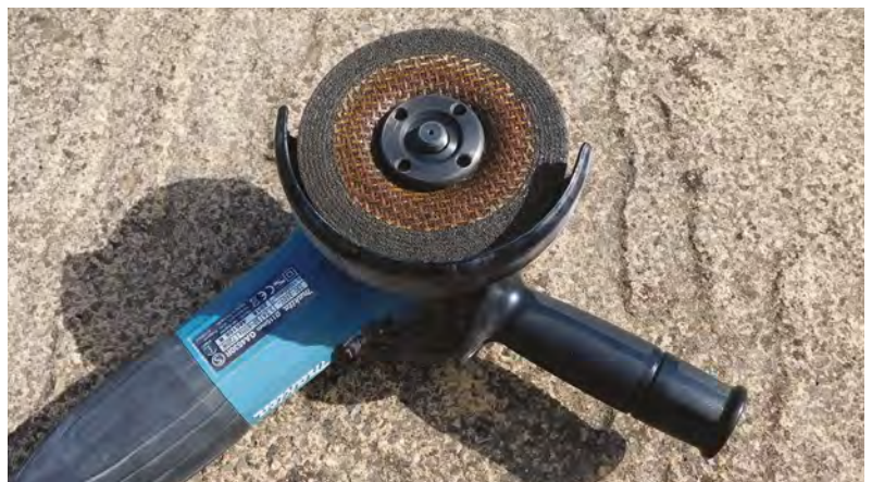
Below ♦ Angle grinders are simple tools: the only control here is the 'on' button
