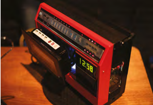
Above ♦ The Pi VCR brings a Raspberry Pi and a flat screen into the body of an old video recorder
